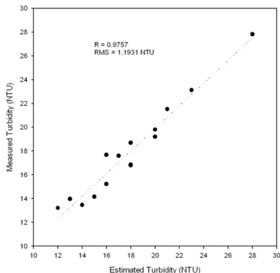
Fig. 5 Relationship between measured and predicted turbidity
