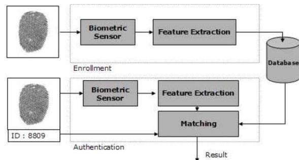
Fig. 6 Fingerprint Verification System
