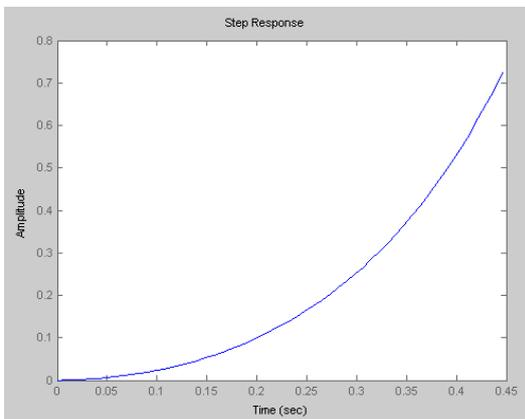
**Fig. 3** Open loop response of Inverted Pendulum represented by eq. (3)
