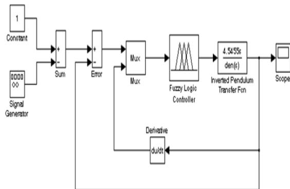
**Fig. 8 MATLAB SIMULINK Model for FLC based Inverted Pendulum**
