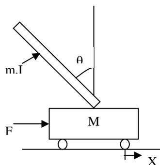
**Fig.1** Model of an inverted pendulum
