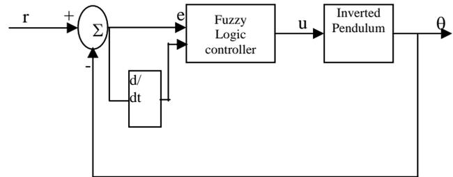
**Fig. 4** Fuzzy Logic Controller for an inverted pendulum on a cart
