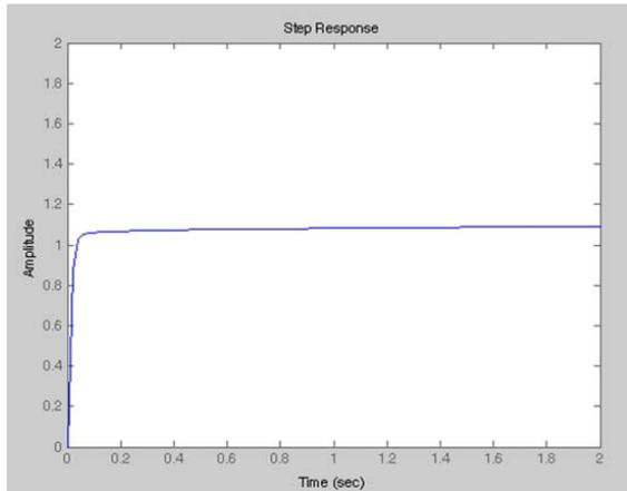
**Fig.6 Output Response of Fuzzy Logic Controller based Inverted Pendulum**
